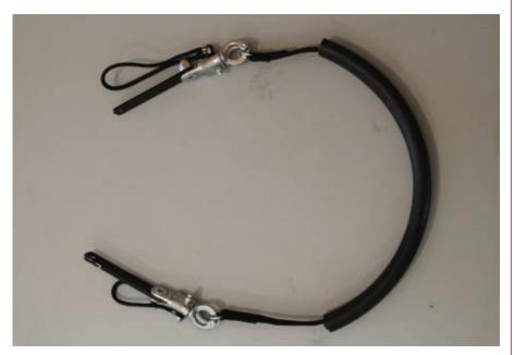
Photo 2: A closer look at the quick-release hardware and system with the rubber hose added to the webbing strap.
